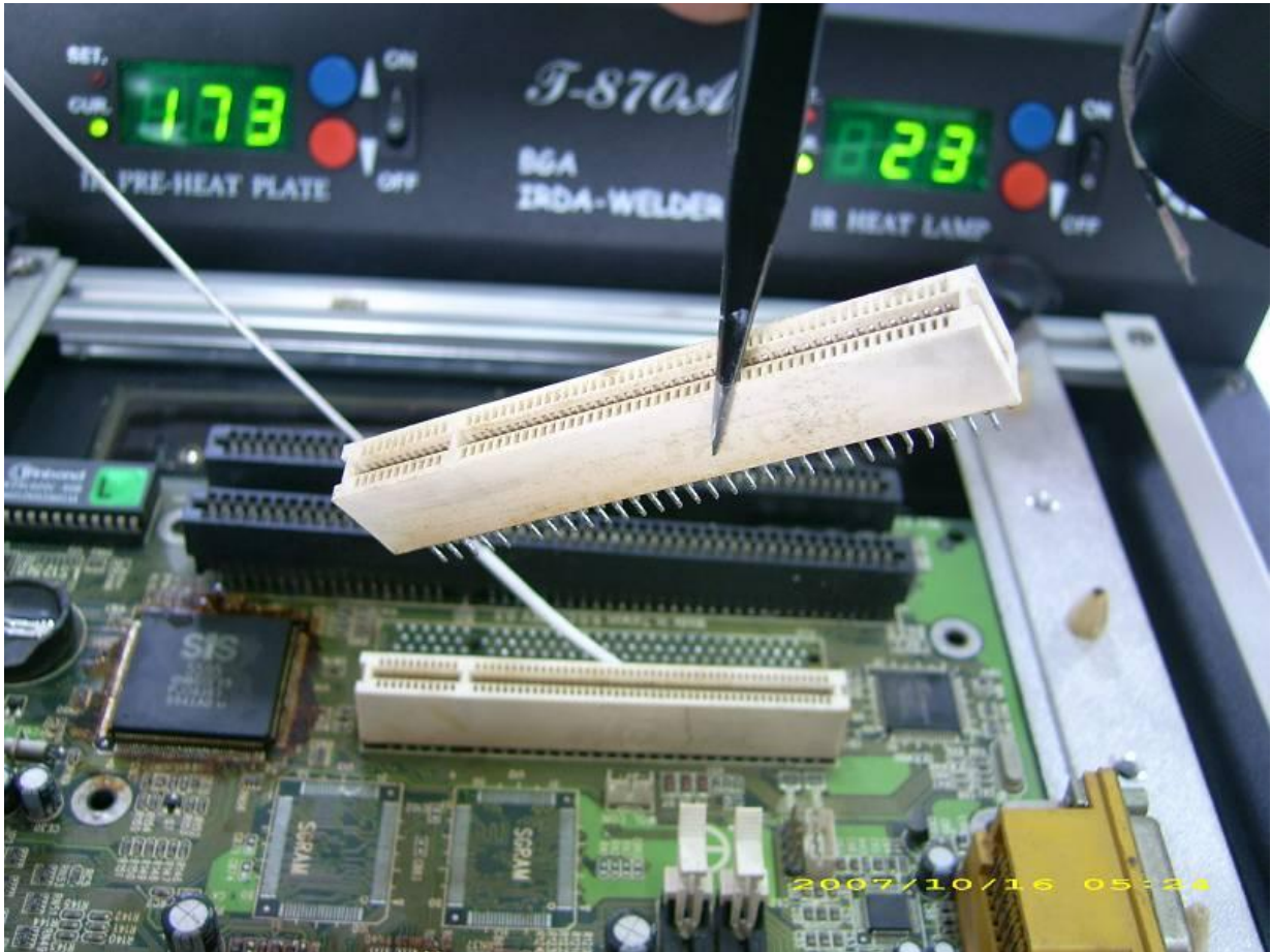
Removal of GAP slot
